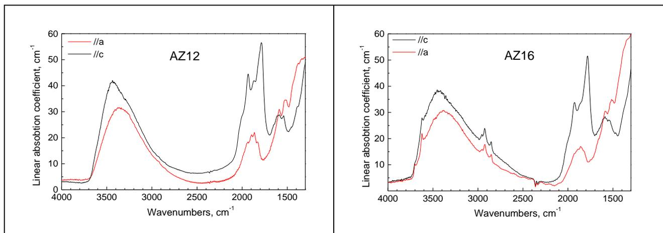
**Figure 3.** IR spectra of different zircon crystals from dykes AZ12 (left) and AZ16 (right) in 4000 – 1300  $\text{cm}^{-1}$  range in polarized light.
