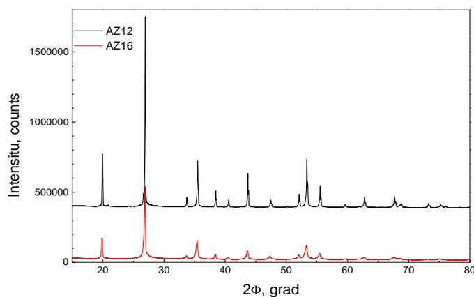
**Figure 2.** Diffractograms of the two zircons.
